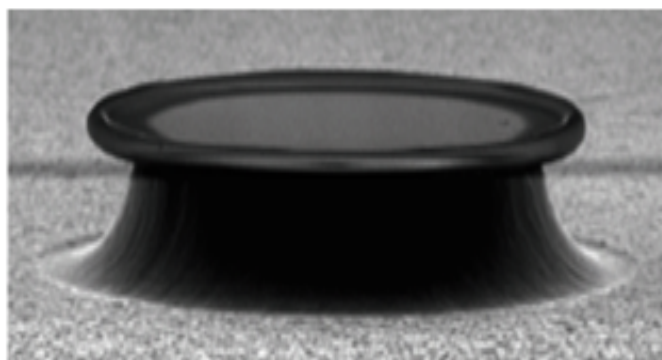
Figure 6: SEM image of a silica microdisc [36].
